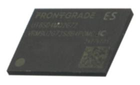
For space applications demanding ultra-high memory density and throughput with exceptional space grade assurances, FRONTGRADE offers the industry leading 18Gbyte DDR4 DRAM memory module. The 18GB DDR4 provides a 2G addressing depth with a 64-bit data plus 8-bit ECC bus width capable of 2400 MT/s data throughput.
