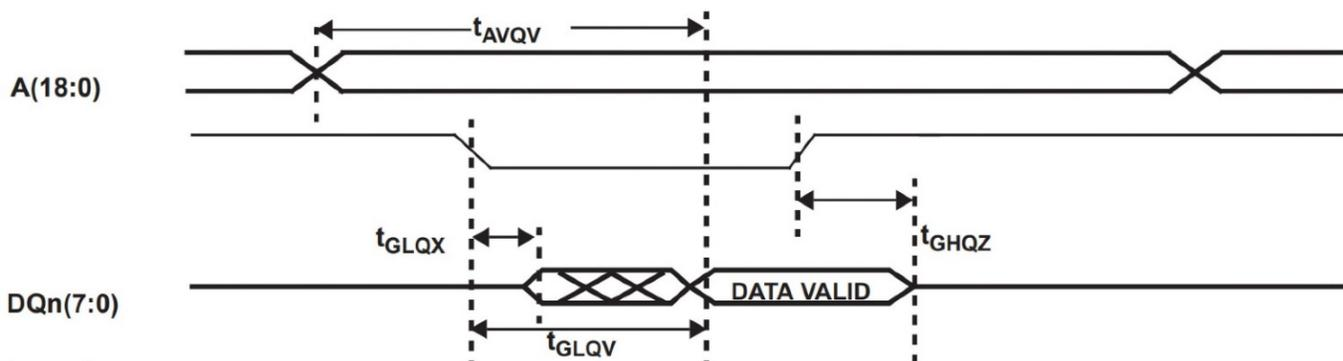
Figure 4c. SRAM Read Cycle 3: Output Enable-Controlled Access
