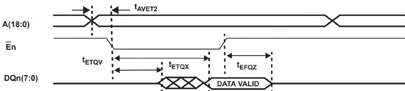
Figure 4b. SRAM Read Cycle 2: Chip Enable-Controlled Access
