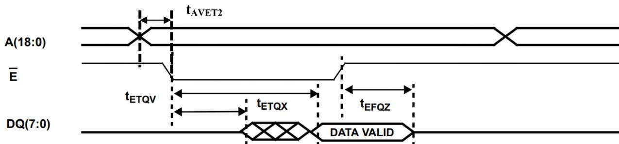
Figure 4b. SRAM Read Cycle 2: Chip Enable-Controlled Access
