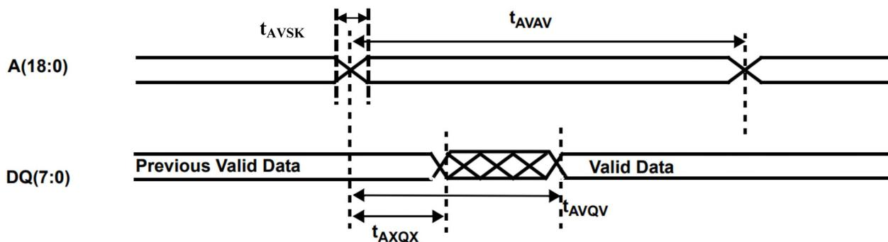
Figure 4a. SRAM Read Cycle 1: Address Access
