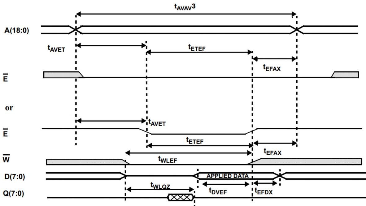
Figure 5b. SRAM Write Cycle 2: Chip Enable - Controlled Access
