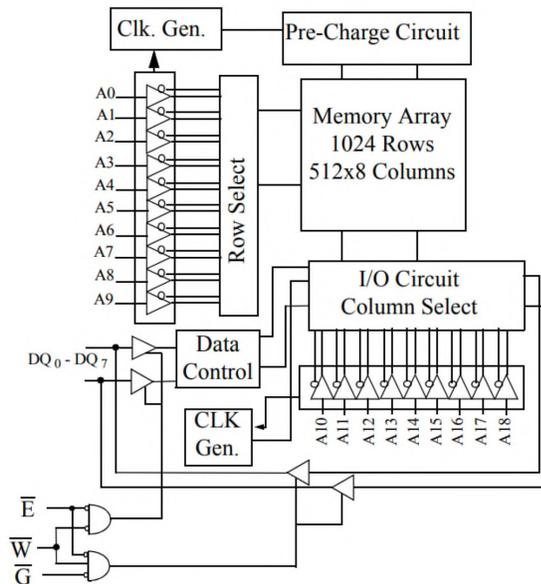
Figure 1. UT9Q512E SRAM Block Diagram
