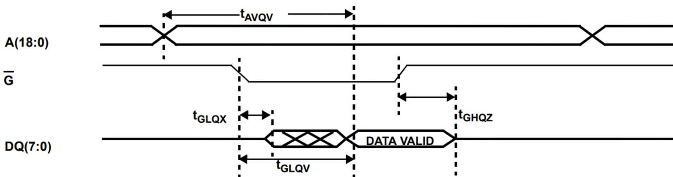
Figure 4c. SRAM Read Cycle 3: Output Enable-Controlled Access
