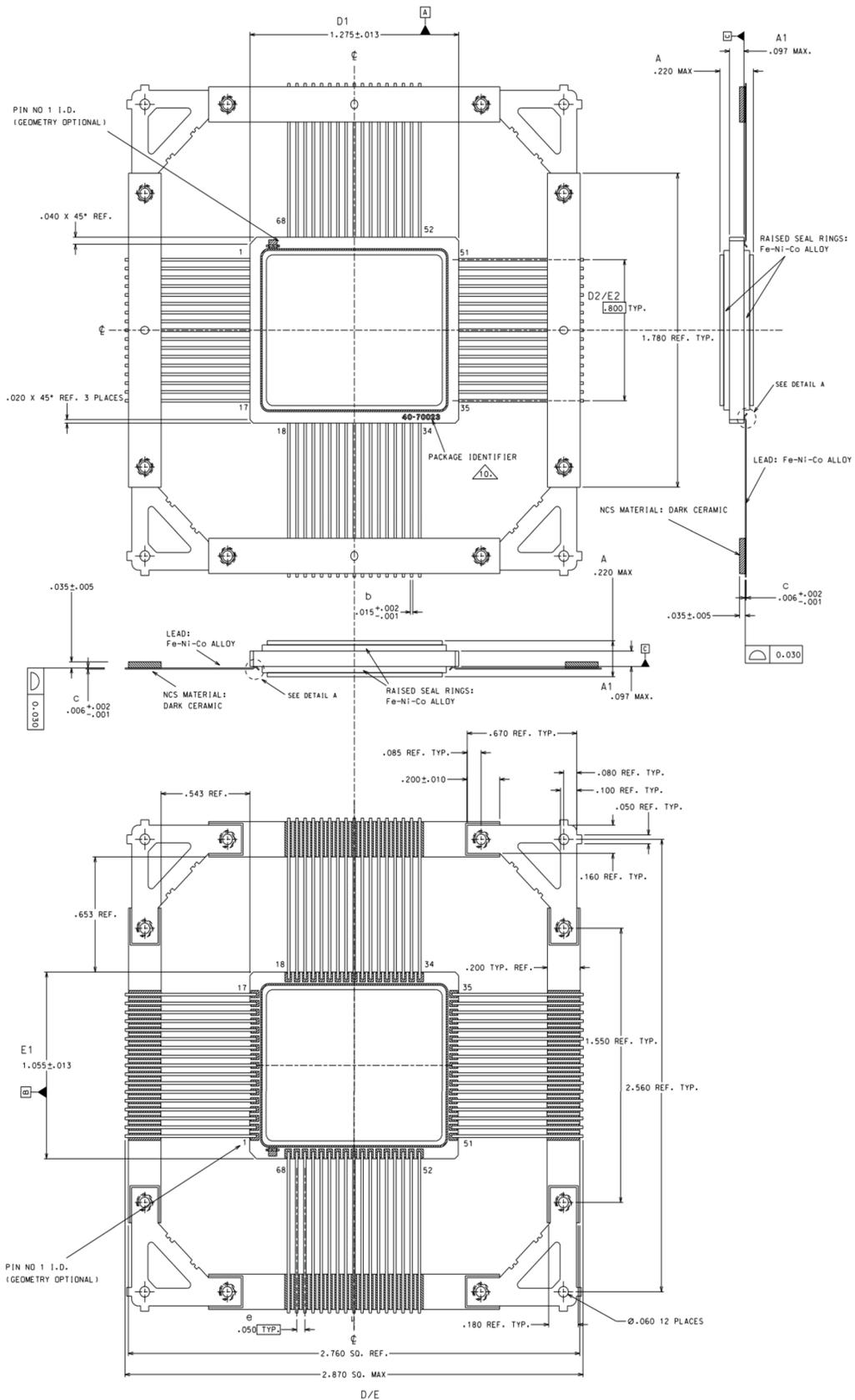
Figure 7. 68-pin Ceramic FLATPACK
