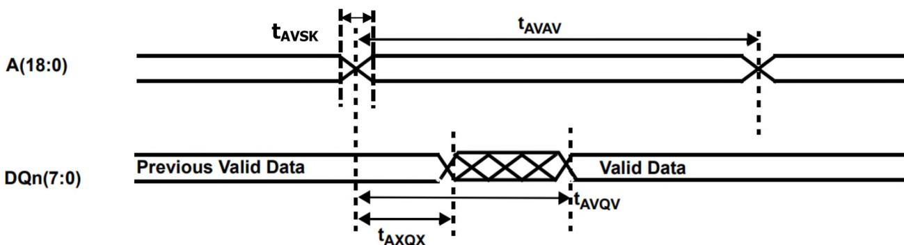
Figure 3a. SRAM Read Cycle 1: Address Access
