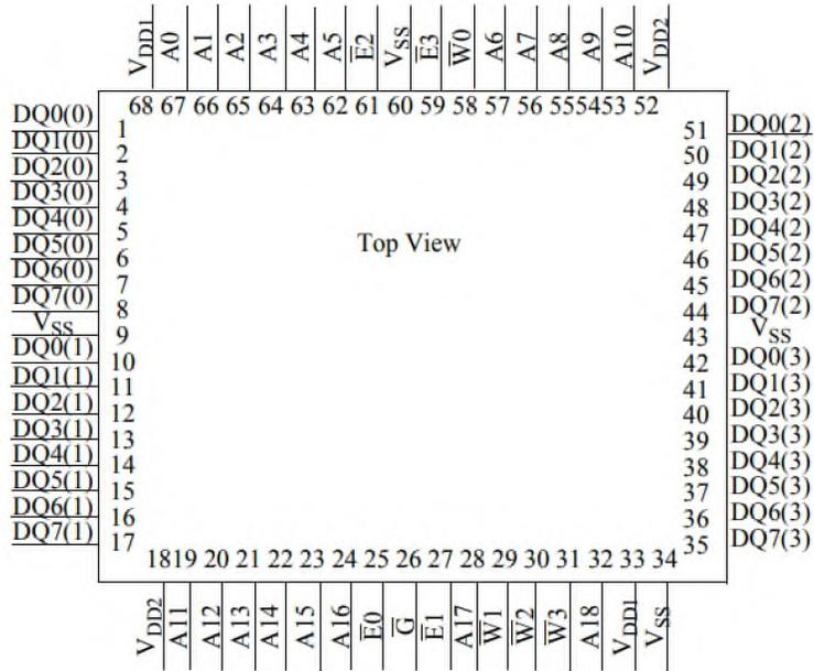
Figure 2: 17ns SRAM Pinout (68)
