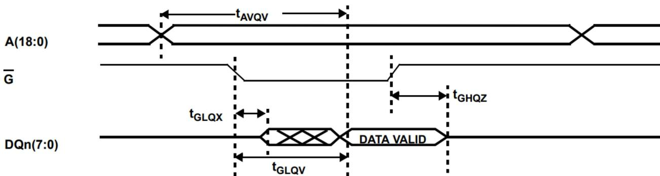
Figure 3c. SRAM Read Cycle 3: Output Enable Access
