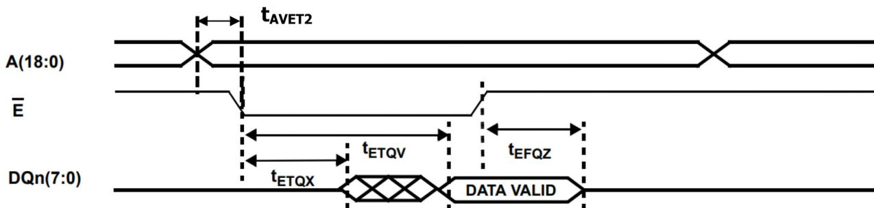
Figure 3b. SRAM Read Cycle 2: Chip Enable Access
