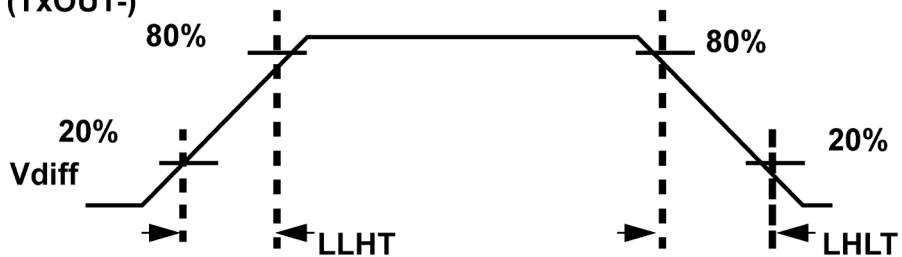
Figure 5. UT54LVDS217 Output Load and Transition Times
