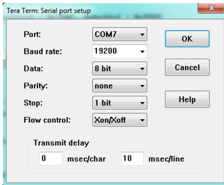
Figure 4: Serial Port Upload Settings
