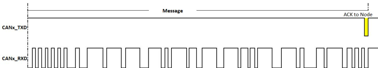
Figure 12: BasiCAN receiving message from a Node
